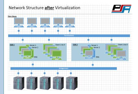
The previously redundant system is now mapped twice to 2 ESXi hosts. Active on ESXi host 1
